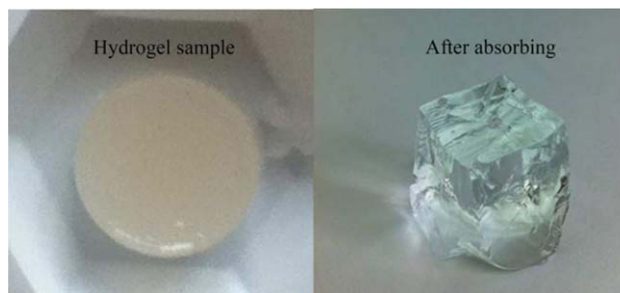
Figure 6. Hydrogel sample and after water absorbing. [Color figure can be viewed in the online issue, which is available at wileyonlinelibrary.com .]
